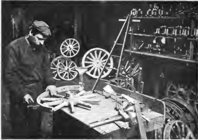
PLACING WOOD RIM IN POSITION ON SPOKES.
